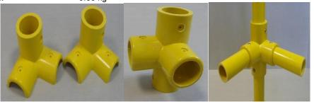
Used to make a 4 way 90deg joint between handrail and stanchion post. The stanchion post must be a continuous length from base to handrail. Knee rail tubes cut to length to fit between adjacent stanchion posts.
