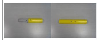
A 300mm length of tube 38mm od to form a joint between lengths of handrail tube. The joint between the tubes is secured with 2 No bolts. Note that the bolts required for this fitting at 45mm long (standard bolt set is 60mm long)
