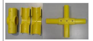
Used to make a 90deg connection (Cross) of the knee rail tube to the stanchion post. The stanchion post must be a continuous length from base to handrail. Knee rail tubes cut to length to fit between successive stanchion posts
